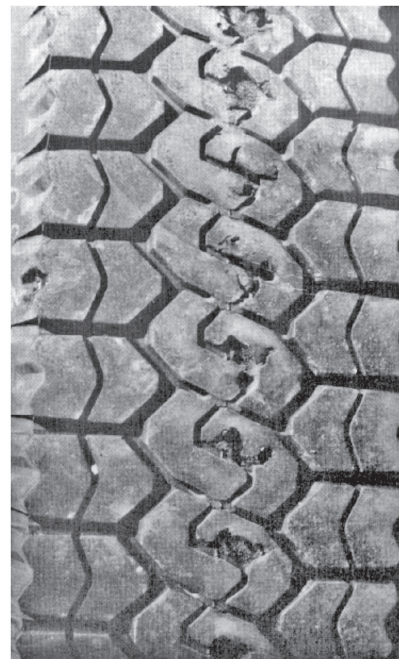
Example of Dyno Damage
